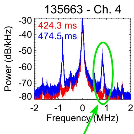
Density fluctuation power in 0.5-1MHz frequency band increases strongly at beam step
